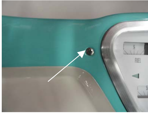
Picture showing left front mounting bolt
