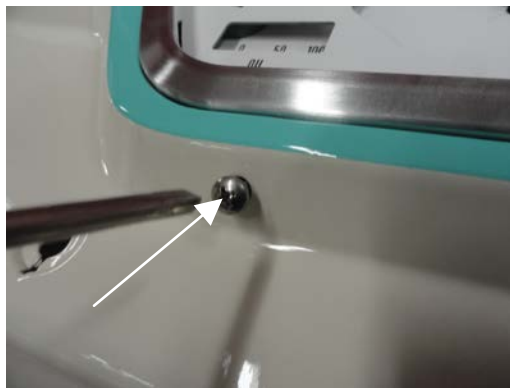
Picture showing bottom left mounting bolt
