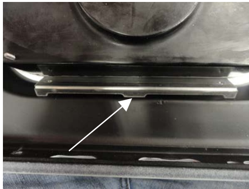
Picture showing bracket placement at bottom rear of gauge cluster
